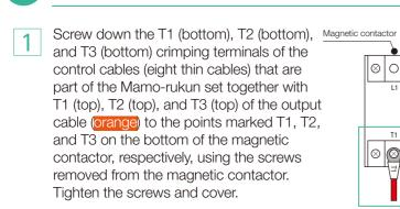
Connect the A1 and A2 crimping terminals to the top of the magnetic contactor and cover.
