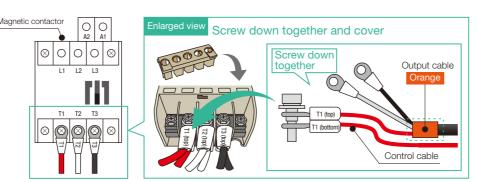
Connect the magnetic contactor (MC) and Mamo-rukun (inrush current protection device) with the cables
